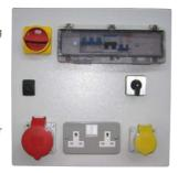
This IP66 enclosure offers both 415v and 110v site supply to IP67 through switched interlock sockets. These are individually protected by RCBOs.
